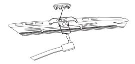
2. Insert wiper arm pin through the correct sized hole in the wiper frame.
