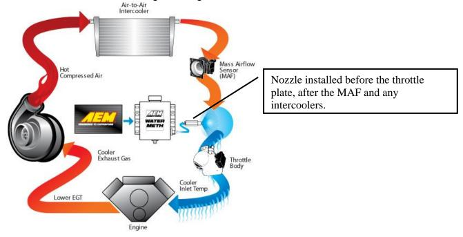
In most instances, the air charge piping can be drilled and tapped for 1/8" NPT to directly mount the nozzle. If using thin walled tubing it's suggested that a bung be welded to the piping. Mounting hole should be tapped deep enough to allow the end of the nozzle to be nearly flush with the interior of the intake once the nozzle is fully installed.
