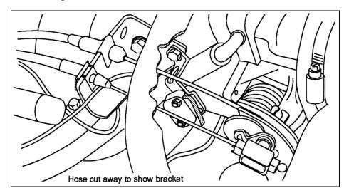
Figure 11 Microswitch Mounting Location—shown at W.O.T.
