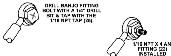
Figure 8 Schematic of "Drilled Out" Banjo Fitting
