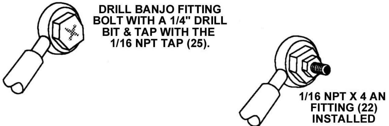
Figure 8 Schematic of "Drilled Out" Banjo Fitting
