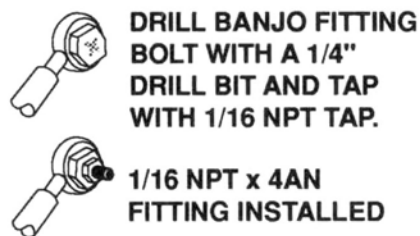
Figure 8 Schematic of "Drilled Out" Banjo Fitting
