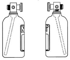
**Figure 4 Nitrous Bottle Mounting Orientations**
