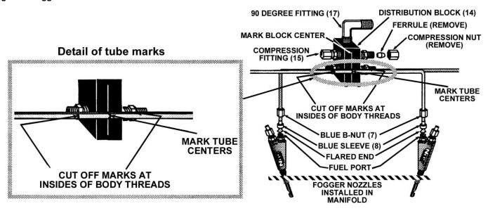
Figure 7 End Fogger Nozzle Feed Tubes
