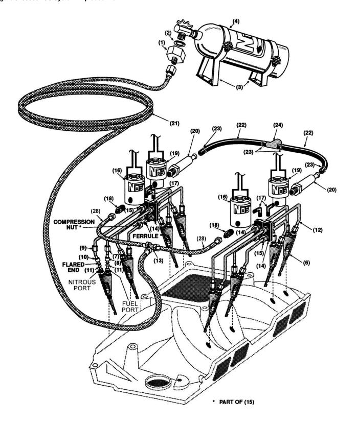
Figure 4 Fogger Nozzle Mounting Position—2x4V Intake
