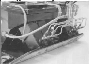
Figure 5 Fogger Nozzle Mounting Position—Single 4V Intake
