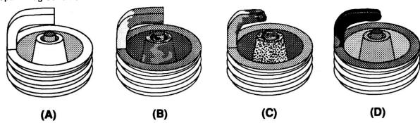
How to Read Spark Plugs form a Nitrous Oxide Injected Engine
