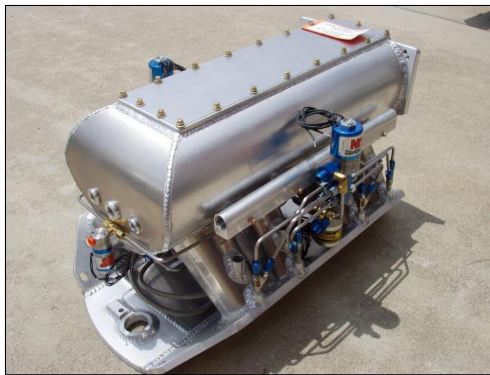
Figure 3 Typical Dry Dual Stage kit installed—Single Plane or Tunnel Ram Intake
