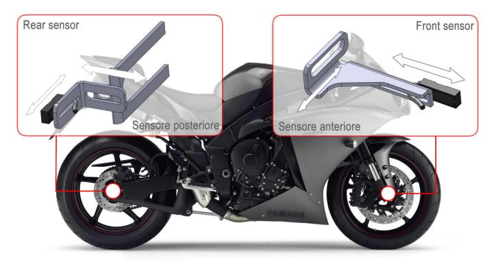
The speed sensors (available for the GRIPONE units) are supplied with a kit of brackets that permit the fitting on the bike. Please follow these steps:
