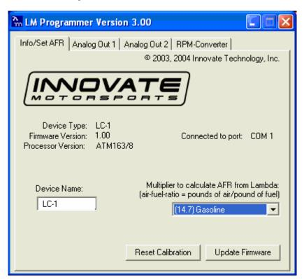
On this page you can see the software version of the LC-1 and you can change the multiplier to calculate AFR from Lambda. A number of different multipliers are already pre-selectable but you can change it to a custom one for the particular fuel you are using.
