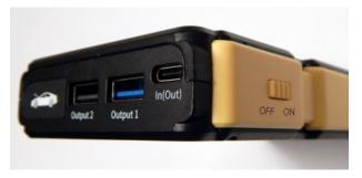
Note the power switch on the side of the unit.
