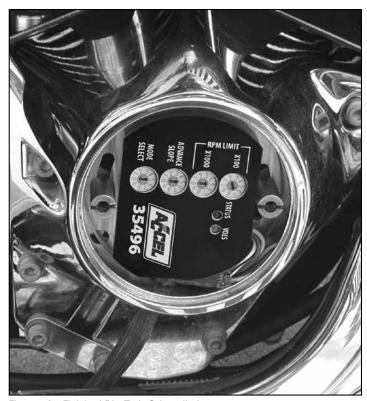
Figure 3A - Finished Big-Twin® Installation
