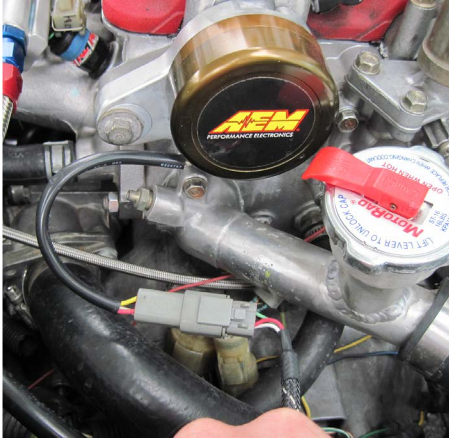
Figure 9. EPM Harness Connected to EPM
