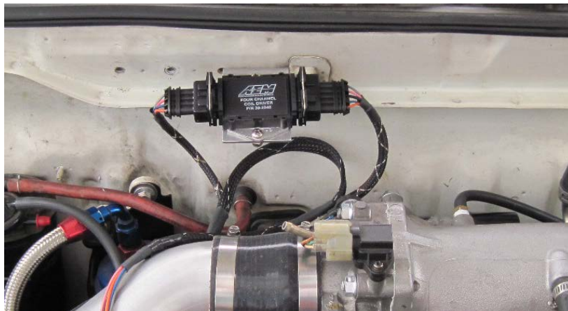
Figure 8. Igniter Mounted and Connected to B Series COP Harness
