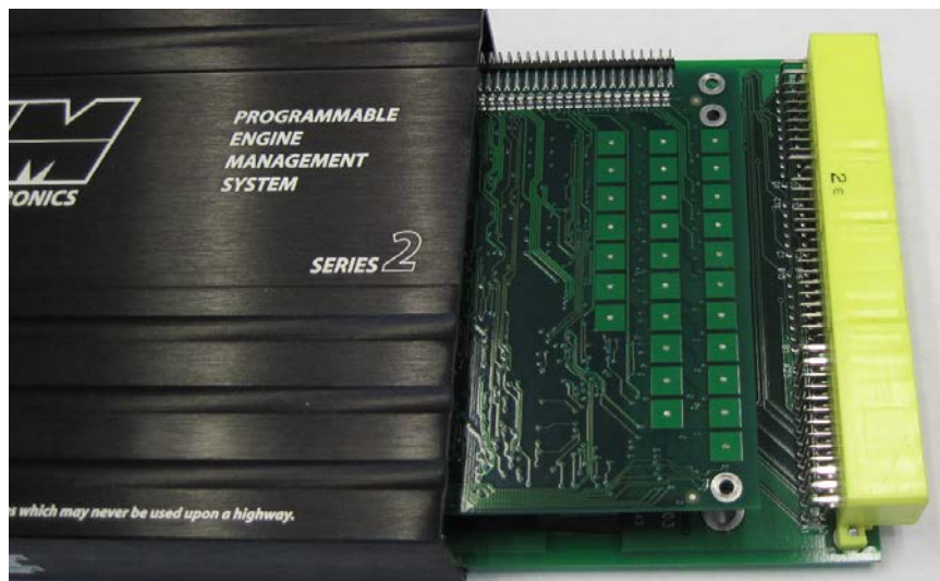
Figure 18. Removing the Circuit Boards
