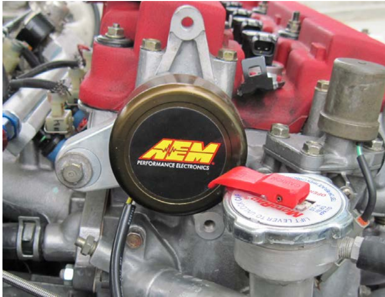
Figure 5. EPM Installed on B Series Engine
