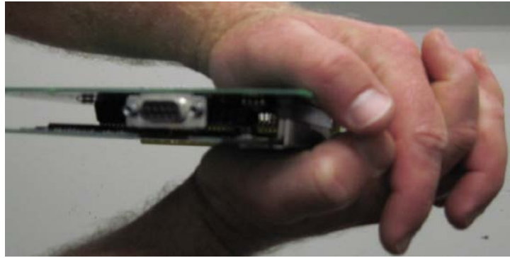
Figure 25. Reassembling the Circuit Boards
