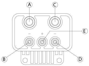
The left and right side of the coil are reversible as long as the stud and the tower are grouped together. For example: tower A/stud B can be wired to fire the rear cylinder and tower C/stud D can be wired to fire the front.
