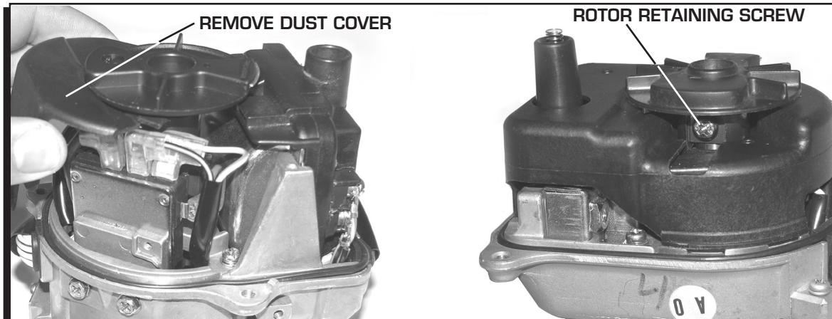
Figure 4 Replacing the Rotor.
