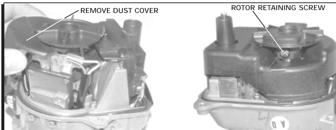
Figure 4 Replacing the Rotor.
