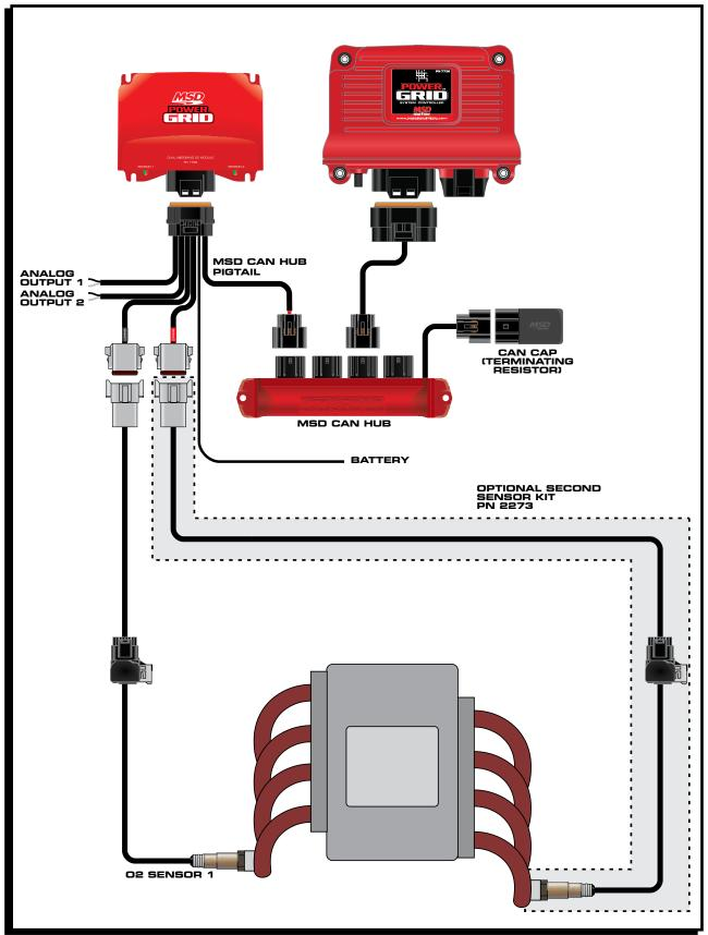
Figure2. MSD Wide-Band 02 Sensor Module System with Power Grid
