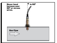
Figure5. 02 Sensor Wire Orientation
