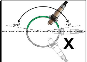
Figure3. Oxygen Sensor Mounting
