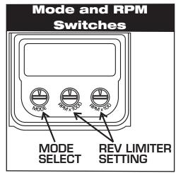
**Figure 2 Mode and RPM Switches**
