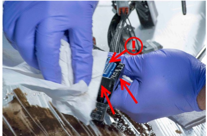
Clean outside of connector housing - avoid terminal openings
