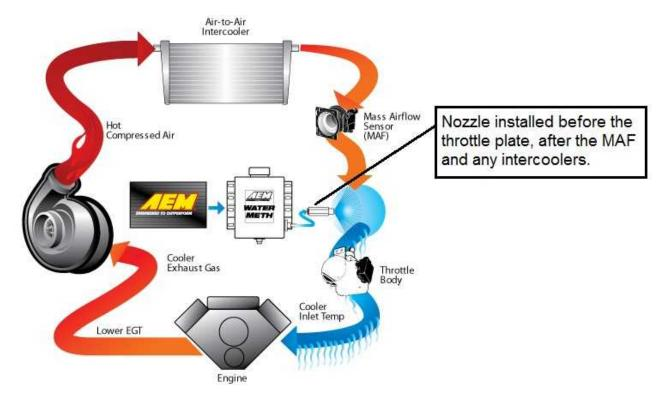
In most instances, the air charge piping can be drilled and tapped for 1/8" NPT to directly mount the nozzle. If using thin walled tubing it's suggested that a bung be welded to the piping. Mounting hole should be tapped deep enough to allow the end of the nozzle to be nearly flush with the interior of the intake once the nozzle is fully installed.
