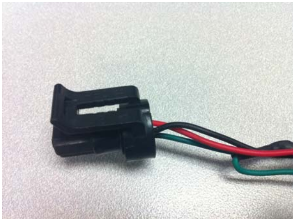
Figure 6. EBP sensor connector
